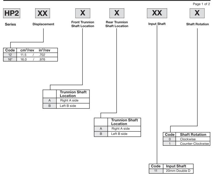
**Note:** Codes are based on pump orientation with "A" & "B" ports on top position as viewed from input shaft end. "Front" pump closest to input shaft end.
