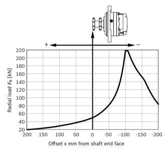
Maximum axial load  $F_{ax max}$  (with radial load  $F_{R}$  = 0):  $F_{ax max}$  = 30700 N  $\leftarrow$  +  $F_{ax max}$  = 25200 N  $\rightarrow$  -
