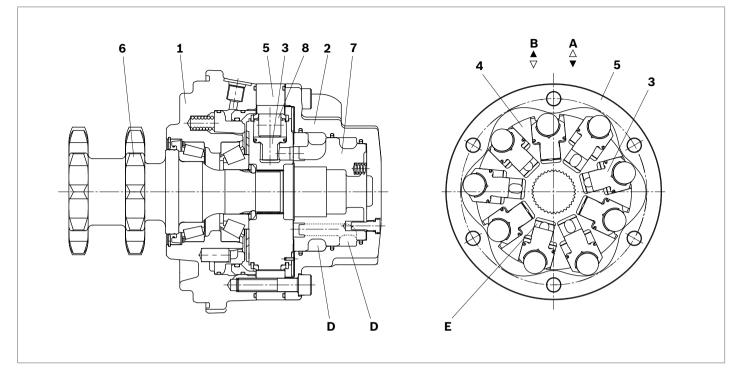
Hydraulic motors, of the type MCR-S, are radial piston motors with front case mounting and sprocket shaft. The MCR-S motors are intended for open or closed circuit operations as drive motors for chain drive functions. The MCR-S motor has the potential to be used in a wide range of applications such as municipal vehicles, agricultural and forestry machines however, the main application for this motor is skid steer loaders.
