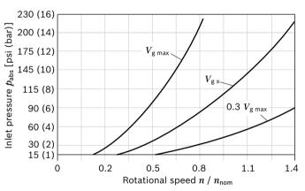
This diagram is valid only for the optimum viscosity range from  $v_{opt}$  = 170 to 73 SUS (36 to 16 mm<sup>2</sup>/s). Please contact us if these conditions cannot be satisfied.
