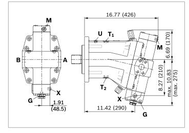
EP.D, EP.P – Proportional control, electric with pressure control fixed setting; remote controlled (EP.G)
