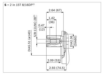
Involute toothing acc. to ANSI B92.1a, 30° pressure angle, flat root, side fit, tolerance class 5
