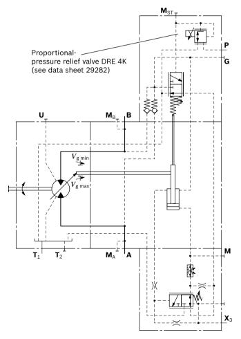
16 **A6VM series 63** | Axial piston variable motor HZ – Two-point control, hydraulic
