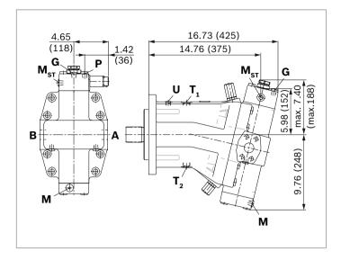
HD.D, HD.G – Proportional control hydraulic with pressure control fixed setting; remote controlled (HD.G)I
