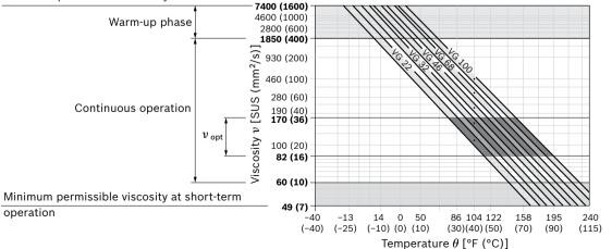
Corresponds e.g. with VG 46 a temperature range of +39 °F to +185 °F (+4 °C to +85 °C)(see selection diagram)
