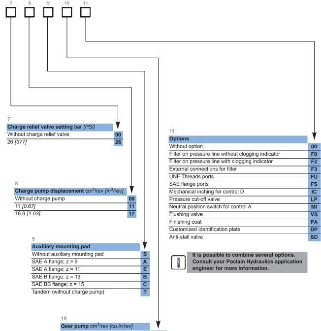
00 Without gear pump 4,0 [0.24] 04 6,0 [0.37] 06 8,5 [0.52] 80 11,0 [0.67] 11 SAE-A flange 14 [0.85] 14 (if digit 9 = A) 16,5 [1.00] 17 19,5 [1.19] 20 22,5 [1.37] 22
