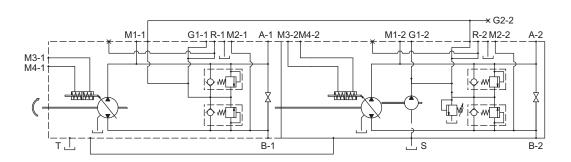
Ports T and G of the first pump must be connected with ports T and G of the second pump.
