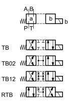
Type **TB\***: 1 solenoid side B 2 positions with return spring
