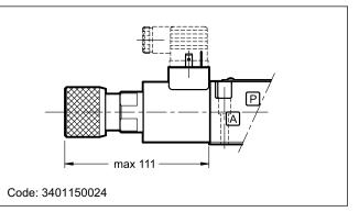
13.6 - CK2-DS3/11 Push and twist manual override (only for DC solenoid valve)
