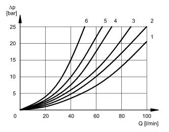
Refer to curve 5 for the pressure drops between working lines A and B of the spools S10, S20, S21, S22 and S23 used in regenerative schemes.
