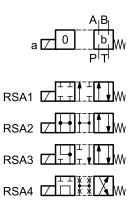
1 solenoid side B 2 positions (central + external) with spring centering рДр SB1 W SB2 SB3  $\overline{\}$ Ŵ W SB4 Type RSB\*: 1 solenoid side B 2 positions (external + central) with return spring 0 Δb
