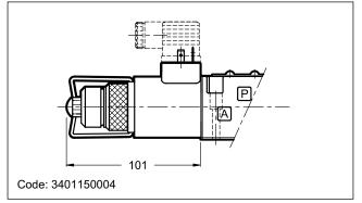
13.4 - CK1-DS3/13 knob manual override, turning (only for DC solenoid valve)
