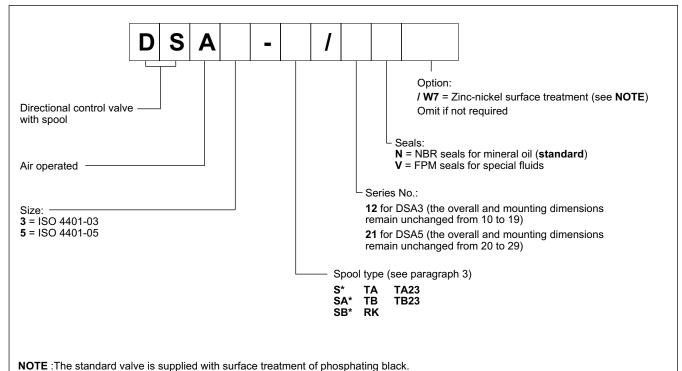
The zinc-nickel finishing on the valve body makes the valve suitable to ensure a salt spray resistance up to 600 hours.
