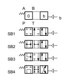
Type **TA**: 1 operation side A 2 external positions with return spring
