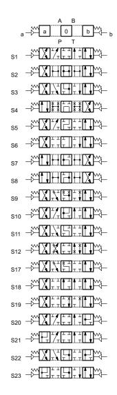
Type **RK**: 2 operations - 2 positions with mechanical retention
