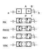
Type **SA\***: 1 operation side A 2 positions (central + external) with spring centering
