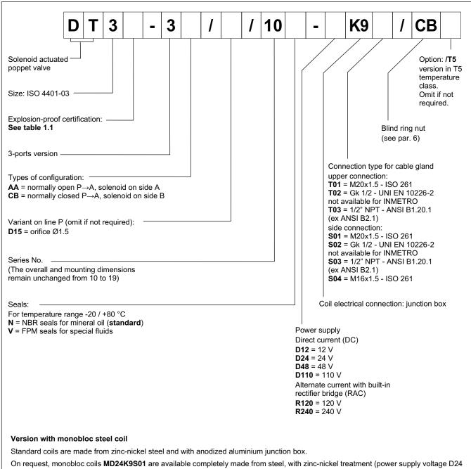
On request, monobloc coils **MD24K9S01** are available completely made from steel, with zinc-nickel treatment (power supply voltage D24 and cable gland connection type S01). Other variants for voltage and cable gland connection are available, always on request.
