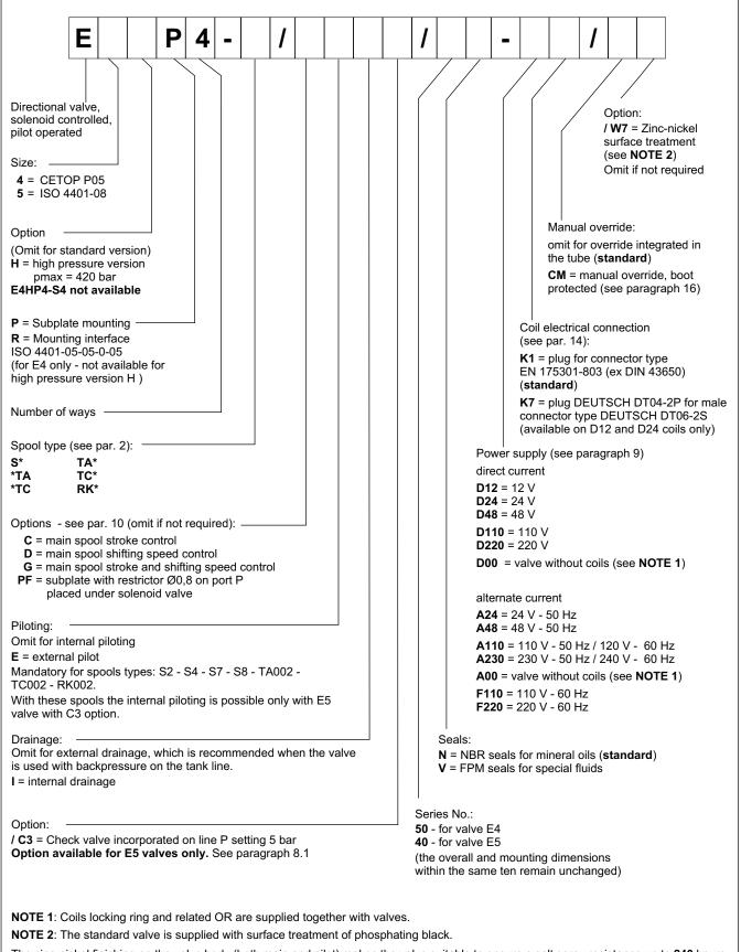
The zinc-nickel finishing on the valve body (both main and pilot) makes the valve suitable to ensure a salt spray resistance up to **240** hours (test operated according to UNI EN ISO 9227 standards and test evaluation operated according to UNI EN ISO 10289 standards). For a salt spray resistance up to **600** hours refer to paragraph 1.1.
