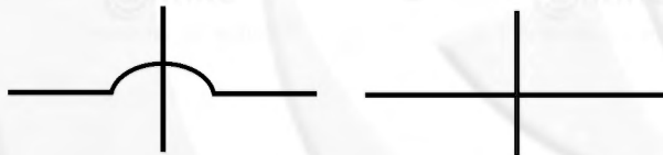
Lines crossing (no connection)
