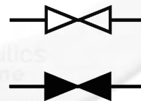
Top: isolation valve (open for normal circuit) Bottom: isolation valve (closed for normal circuit operation)
