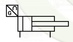
Double-acting cylinder with internal stroke transducer
