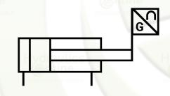
Double-acting cylinder with displacement encoder on piston rod
